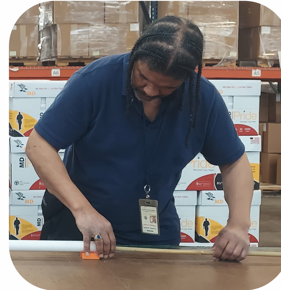
Quality Control Testing Canes are passed through a 1" diameter pipe to check for straightness.
