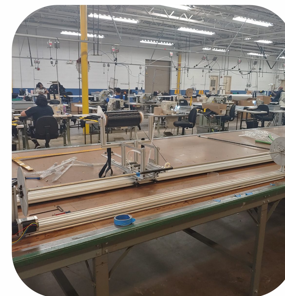
Filament Winding Composite cane shafts are made with an automated winder.
