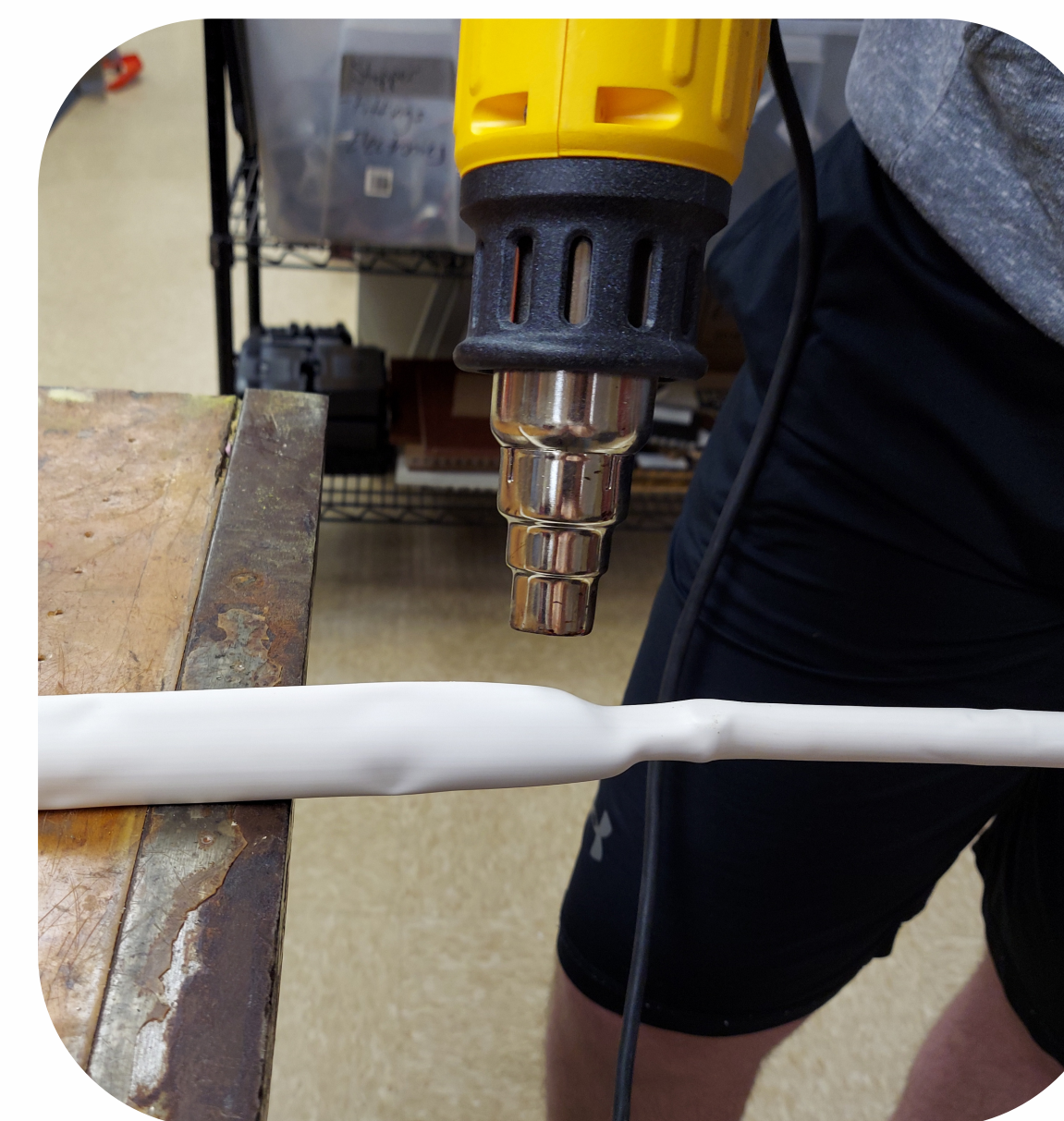
Heat Shrink Tubing Heat shrink is added to the shaft as a sealant and color option.
