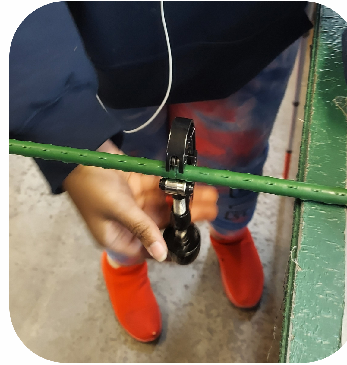
Cane Cutting A pipe cutter is used to cut canes to a desired length (standard lengths are in 2" increments).
