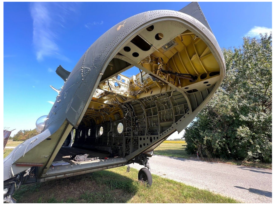
Stripped CH-47 Airframe
