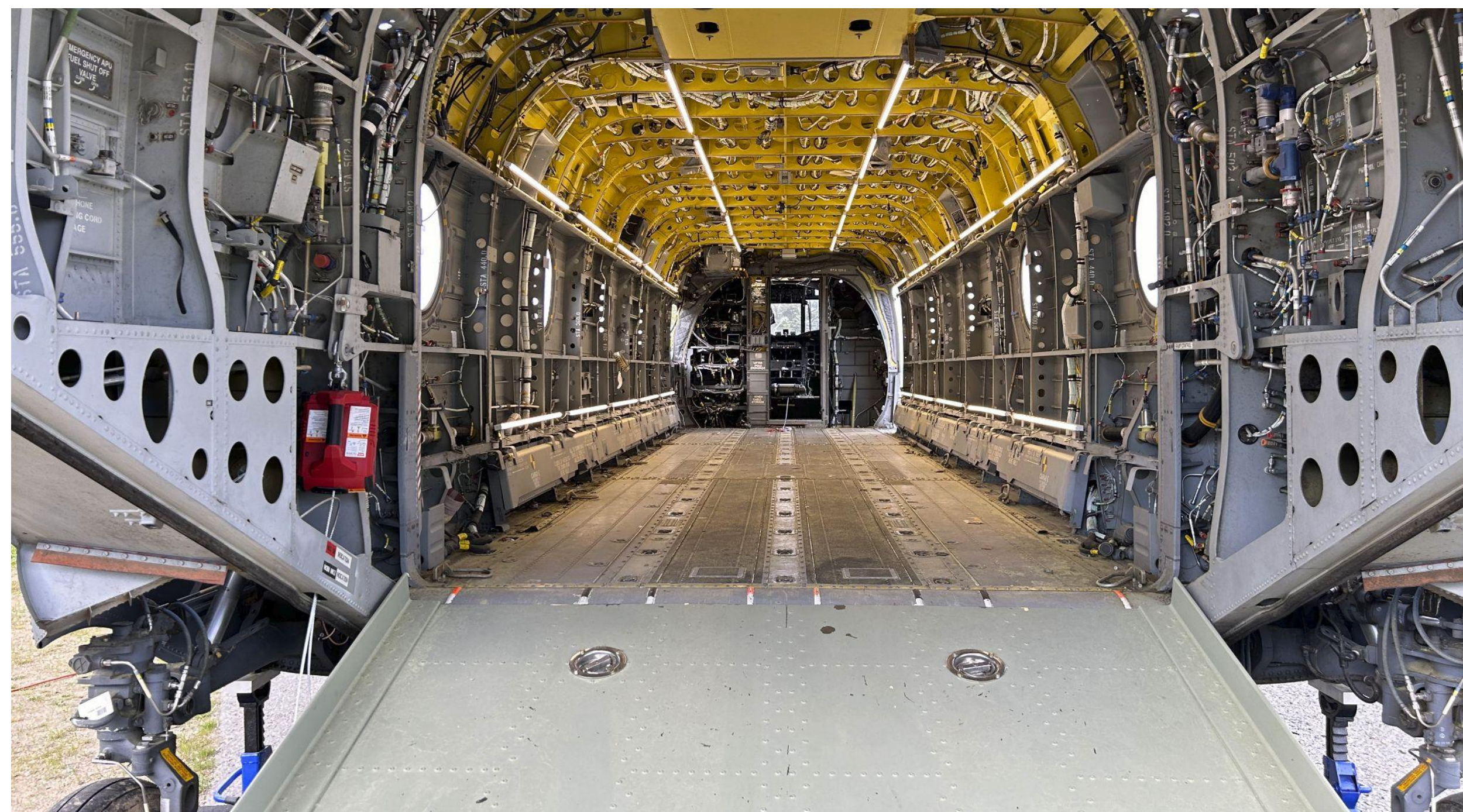
Above: Six courses of LED light fixtures installed in the cargo area
