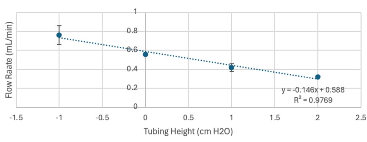
Fig 4. Verification of model to identify tubing height necessary to achieve equal inflow and outflow.
