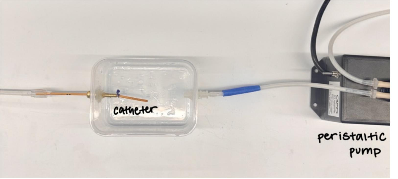
Fig 3. Most recent model prototype, with input flow of 0.6 mL/min.
