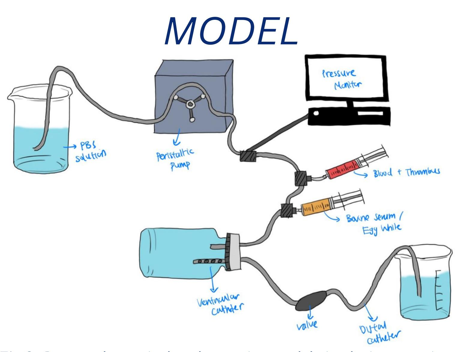
Fig 2. Proposed ventricular obstruction model simulating protein and blood obstruction, with inflow pump and outflow shunt valve.
