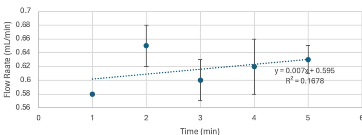
Fig 5. Verification of constant flow through model over five-minute time period.
