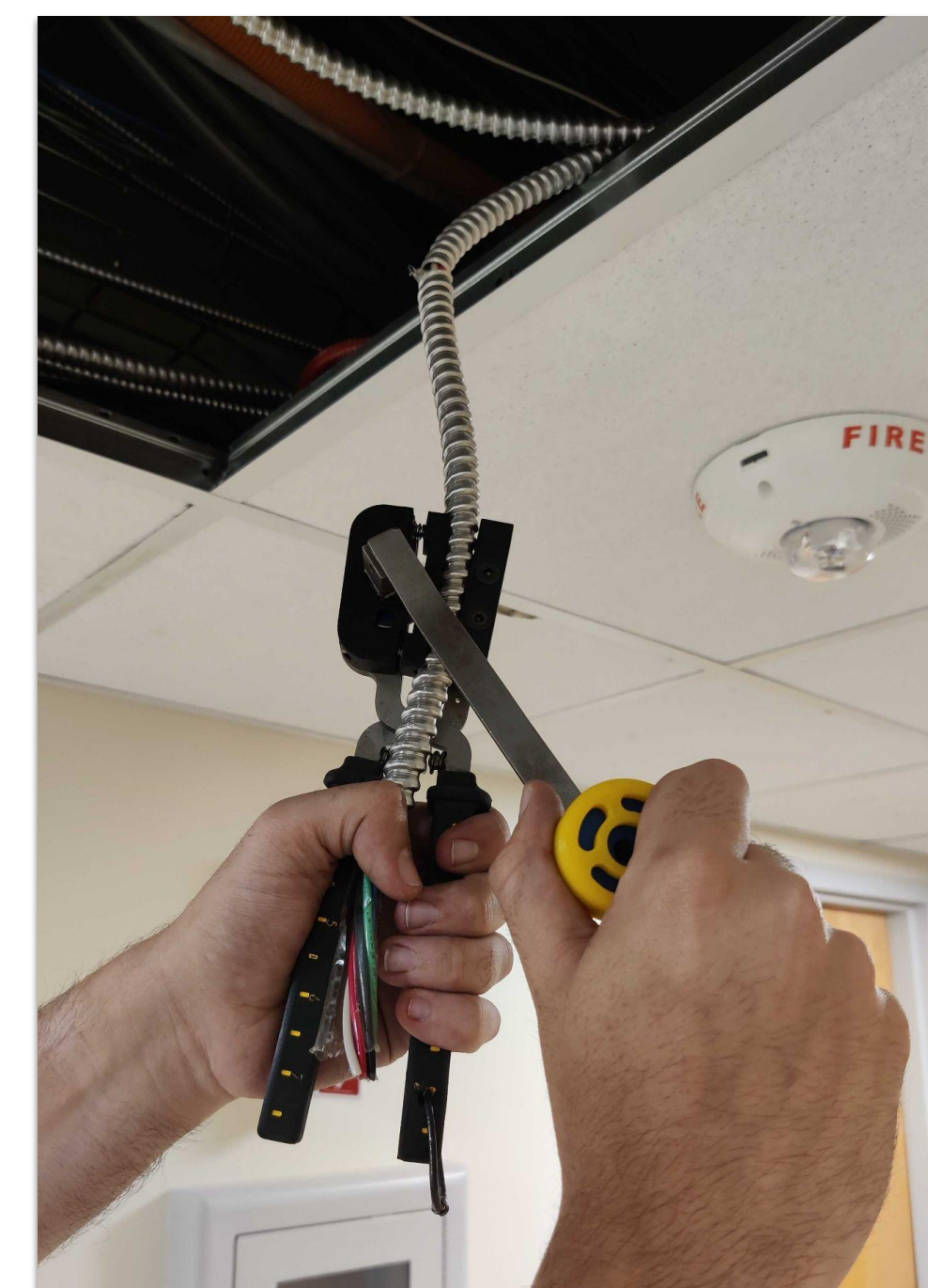
Condu-Cut being used on 3/8" aluminum conduit in a drop ceiling environment.
