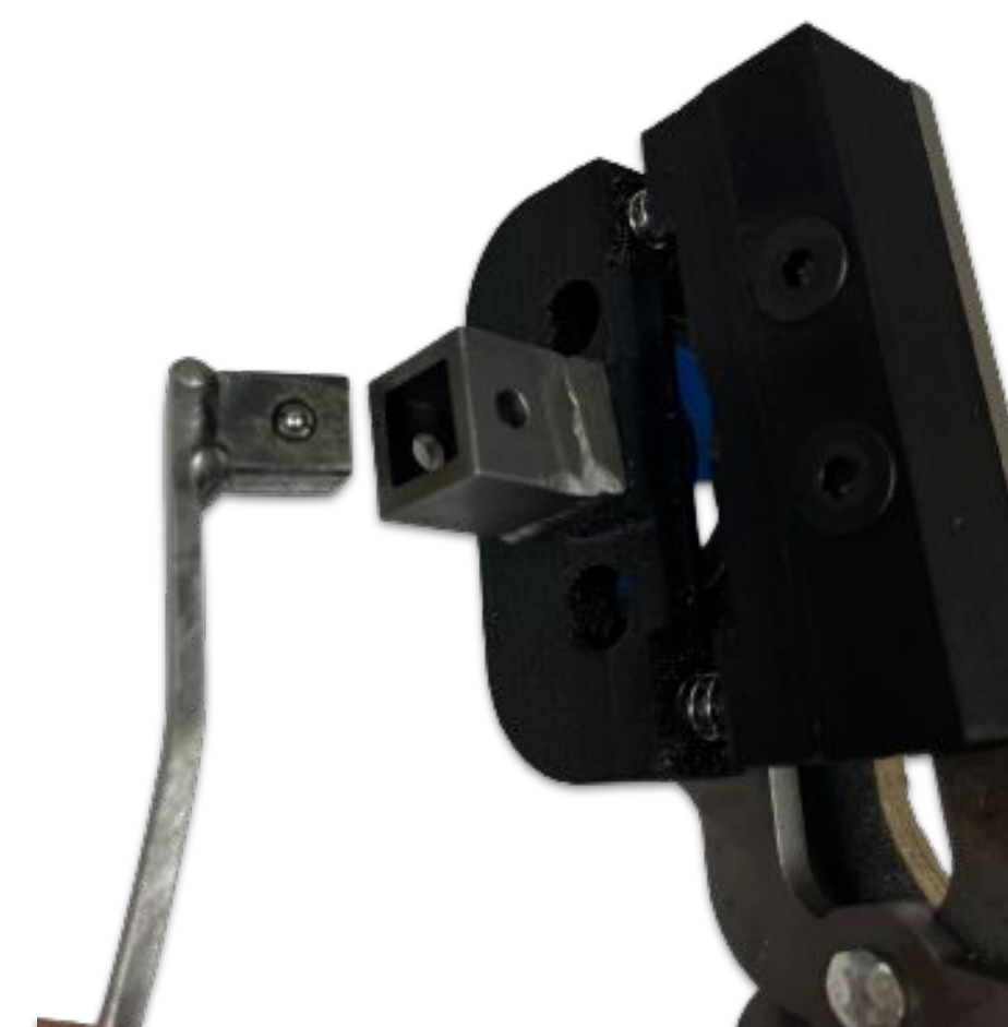
Quick-Release uses a ball-spring plunger and a standard 3/8" female socket.
