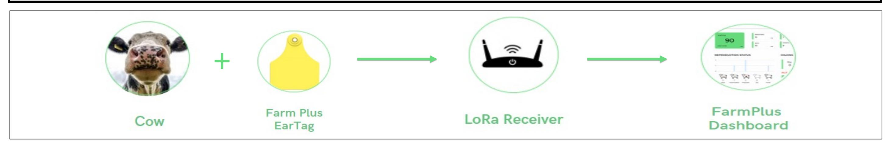
Our Farm Plus Ear Tag has different sensors: Sound, Motion, Temperature to track cow's physiological parameters. The data is received by a LoRa Receiver and sent to the server for storage and analysis. The insights from the data will be available on our dashboard.
