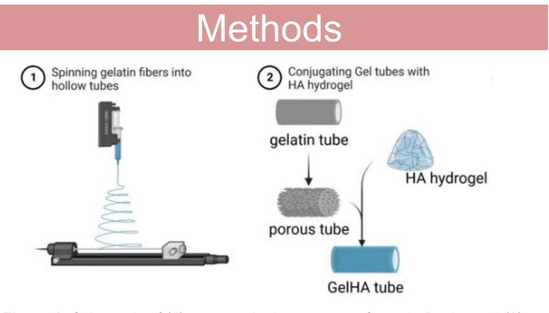
**Figure 2.** Schematic of (1) electrospinning process of gelatin B tube and (2) covalent crosslinking of HA hydrogel with gelatin B tube.
