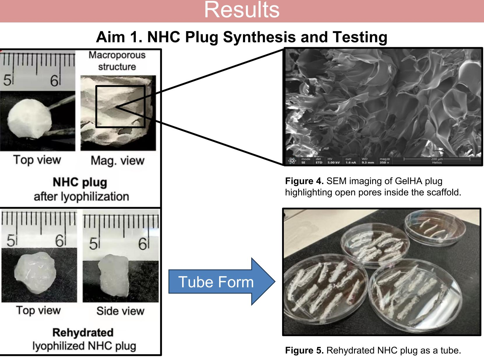
~ 3-fold increase in elastic modulus of NHC plug shows inclusion of gelatin B improved shape retention when compared to the pure HA gel.
