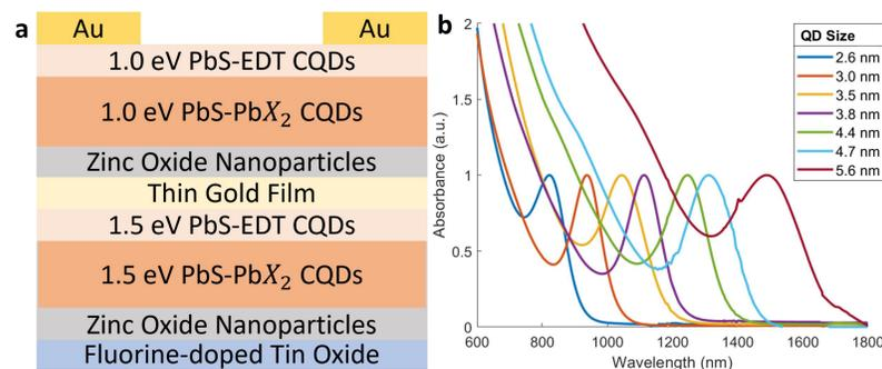
Figure 1. (a) Structure of a tandem CQD solar cell. The thin gold film acts as a recombination layer to enable the flow of charges between both sub-cells. (b) Plot showing the change in absorbance as the diameter of the CQD is changed. CQD sizes calculated based on work by Moreels et al. and absorption peaks observed in the UV-Vis spectra [3].
