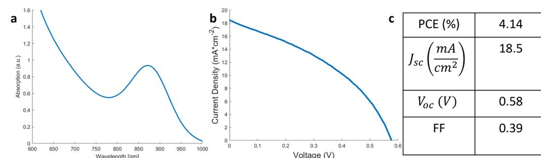
Figure 5. (a) UV-vis spectrum for approximately 1.4 eV (870 nm) CQDs. (b) JV curve for a fabricated 1.5 eV sub-cell and (c) photovoltaic performance parameters for the same cell.
