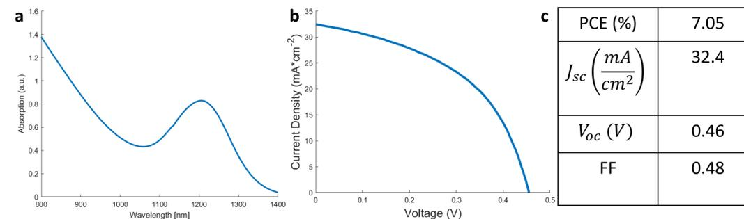
Figure 4. (a) UV-vis spectrum for approximately 1 eV (1210 nm) CQDs. (b) JV curve for a fabricated 1 eV sub-cell and (c) photovoltaic performance parameters for the same cell. PCE = power conversion efficiency;  $J_{sc}$  = short-circuit current density;  $V_{oc}$  = open-circuit voltage; FF = fill factor.
