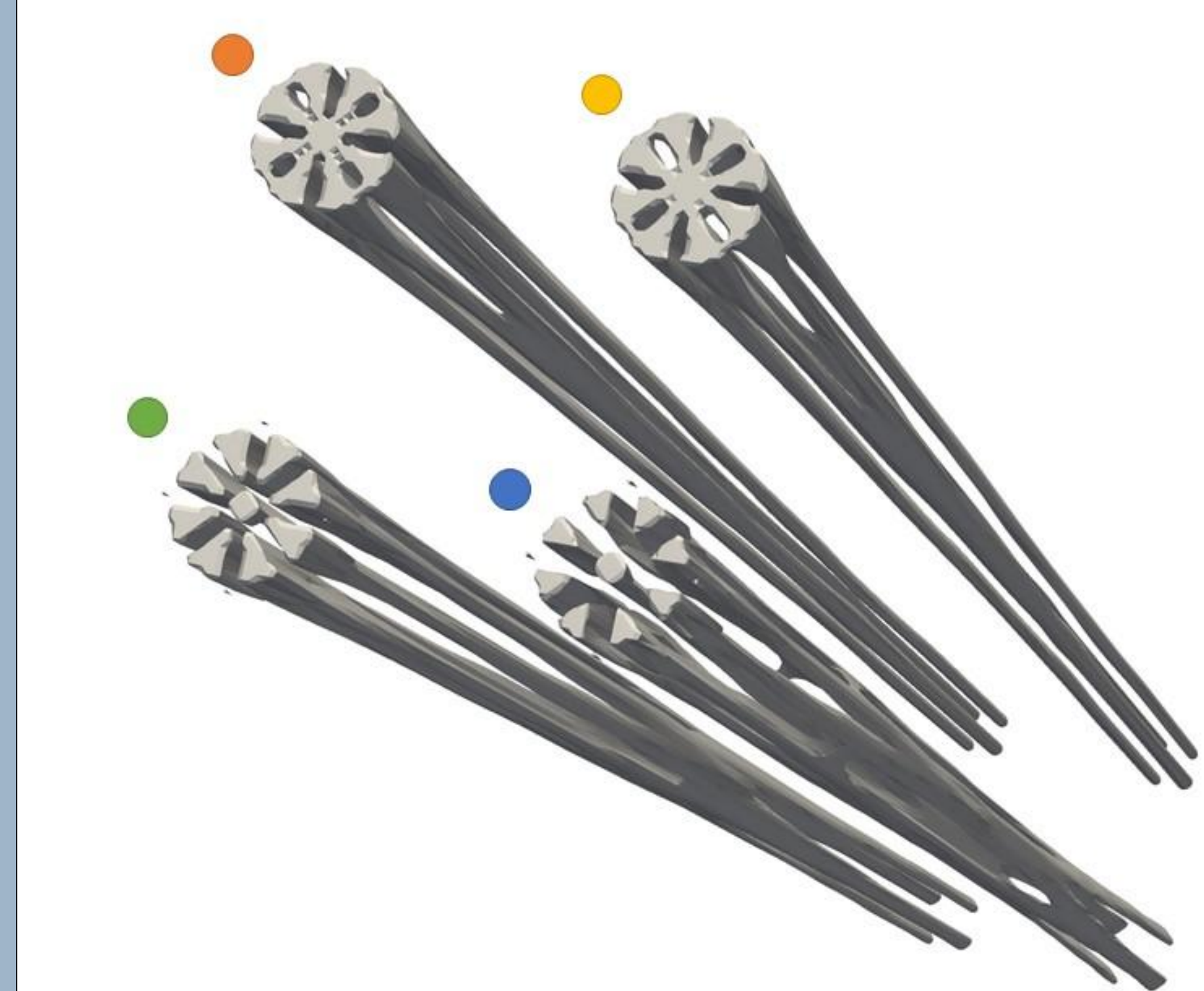
Figure 7: Optimization and corrosion of cylindrical IR generated by MATLAB. Colored dots represent models at various stages of degradation (Orange at 0 months, Yellow at 2 months, Green at 4 months, Blue at 6 months)
