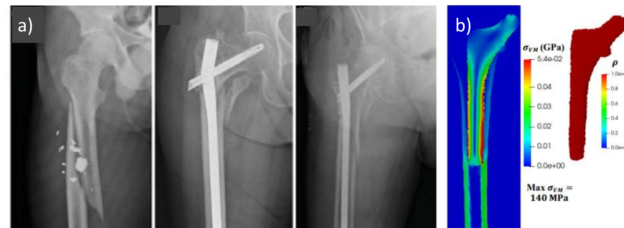
Figure 1: a) Intramedullary rod placed in femur to stabilize fracture. b) Stress map of rod under loading during step.
