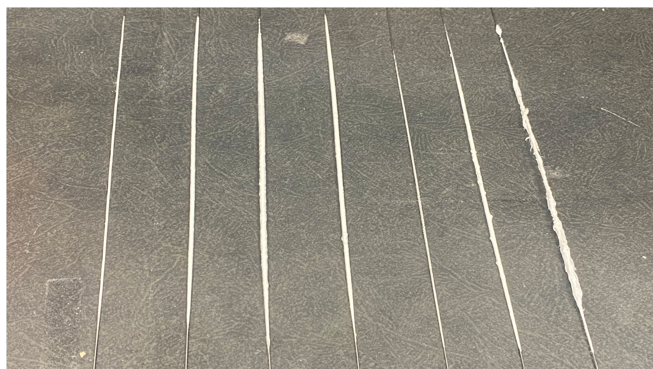
Figure 1. Side by side of different electrospun stainless steel rods of a diameter of 0.0031 in. From left to right, PLA 5%, PLA 8%, PLA 10%, PCL 10%, PLA 5% with 1 w.t. % Vancomycin, PLA 5% with a 4:1 ratio of DCM to Isopropanol with 1 w.t. % Vancomycin, PLA 5% with a 1:1 ratio of DCM to Isopropanol with 1 w.t. % Vancomycin.
