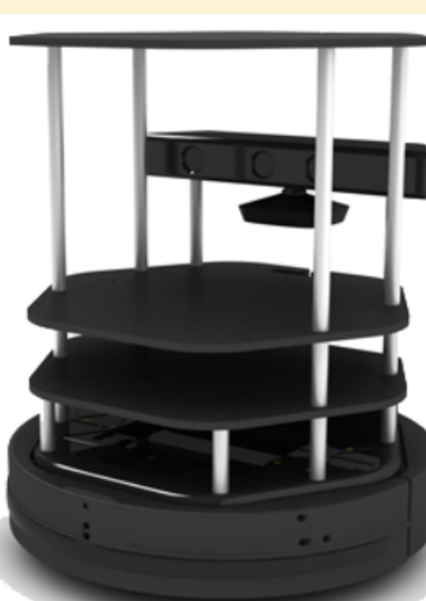
Figure 4. Turtlebot used to begin learning ROS and how to program a robot to move in preparation to code the rover
