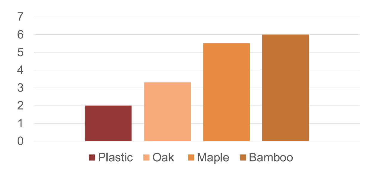
Figure 4: Wood costs. Comparison of cost of different woods as compared to plastic (cost/kg for bulk orders).
