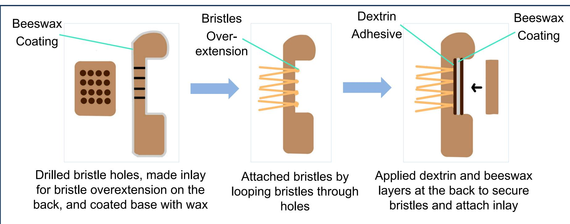
Figure 2: Bristle attachment. Our method of attaching bristles without using any other materials while maintaining strength and durability.
