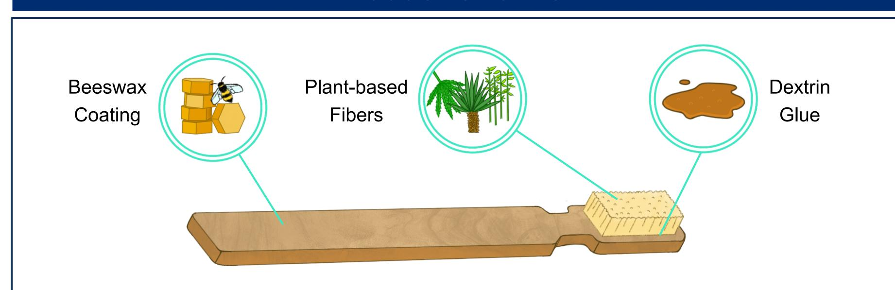
Figure 1: Toothbrush schematic. Our design features waterproof beeswax coating the wooden body, plant-based bristle fibers, and food-safe dextrin glue.
