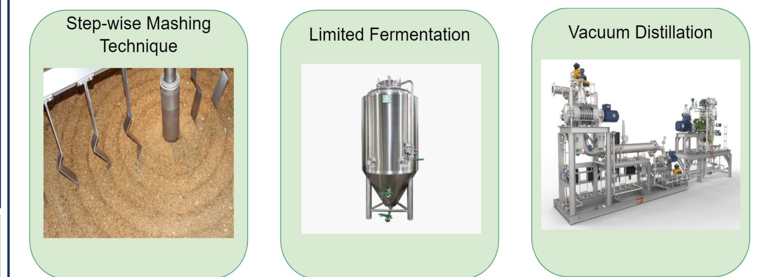
Figure 5 - Manufacturing Highlights Three unique manufacturing process in our beer production: step-wise mashing, limited fermentation using S. ludwigii , and continuous vacuum distillation.
