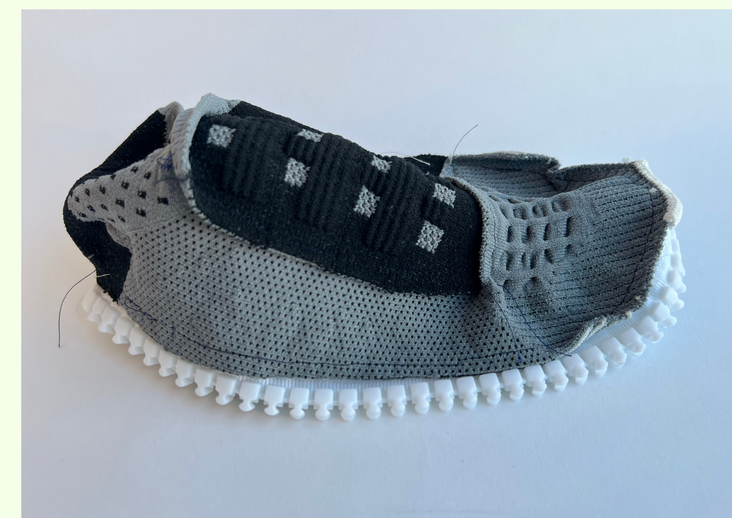
Existing Under Armour™ upper sewn to top half of zipper
